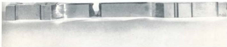
Fig. 6. Fatigue Failure of Specimen from Test With Fretting
