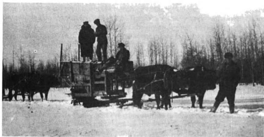
Sweep-operated threshing outfit: Dmytro Rudy's first threshing machine, 1910. (From Hardships and Happiness - Pine River. )
