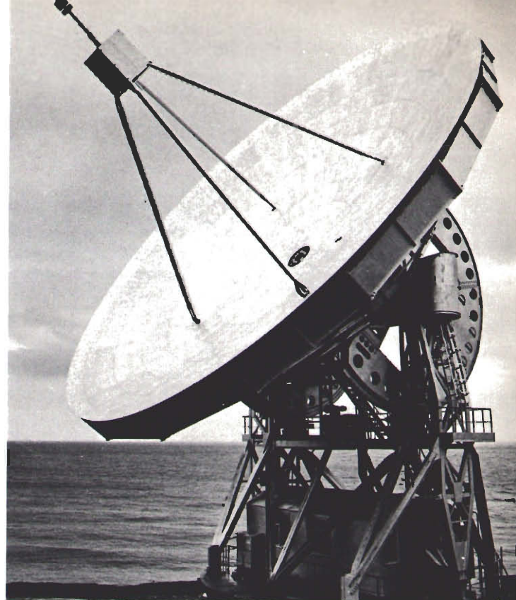
Radio telescope with 72' antenna of Crimean Observatory.
