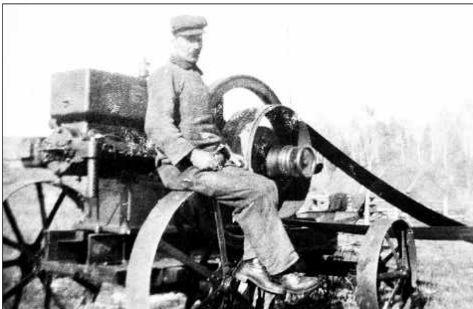
Above: During the early decades a few horse-drawn 'stationary-engines' such as the one depicted above powered threshing machines and saw mills in the district. The self propelled Case steam-engine was more versatile but more expensive to purchase. RTM-033.
