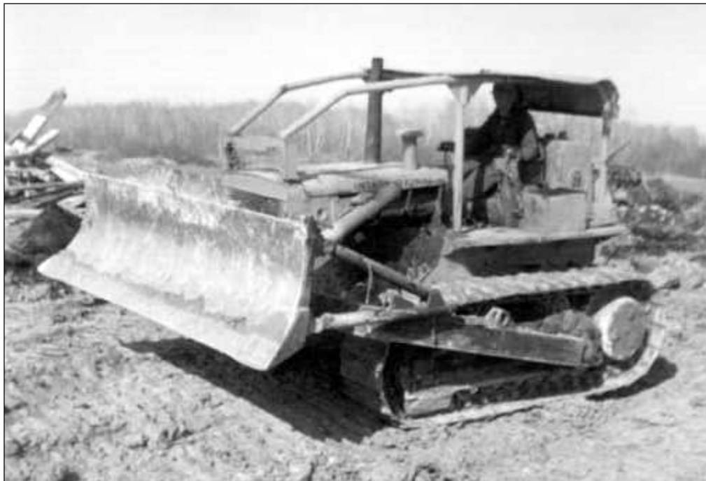
Left: Clearing land in the Poplarfield district with an International TD-A Caterpillar, c1970. Note the heavy crashbar which is fitted to the machine when it is being used to up-end and pile heavy brush. RTM-076.
